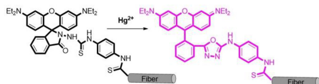
Figure 3. Schematic representation of the cyclization reaction of TEA treated Md-RhB/chitosan nanofibres.
