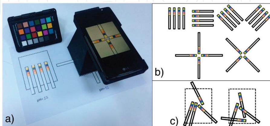
**Figure 4.** The overall smartphone-based colorimetry with apparatus and X-rite ColorChecker passport for color correction are shown in (a). The pH strips with various orientations used in imaging are given in (b), and (c) shows random orientations and positions of the test strips inside the smartphone field of view for dual-illumination tests.
