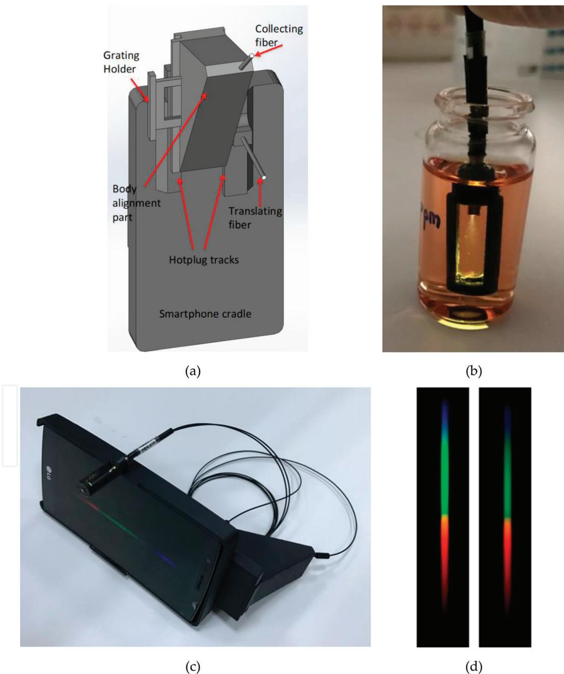
**Figure 3.** (a) The custom-designed cradle for smartphone-based spectrometer. Immersion probe for absorbance measurement is given in (b) and overall design is illustrated in (c). (d) The spectral images obtained from smartphone spectrometer.
