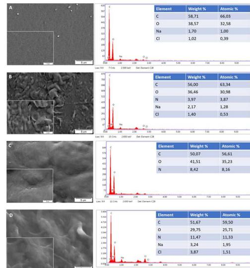
Fig. 3. SEM images and EDX results of PCL membranes. A. Control group, B. PPGCYNTQALEQQ, C. PPGCYNTQALEDDQ, D. PPGCYNTQALEDNQ conjugated membranes
